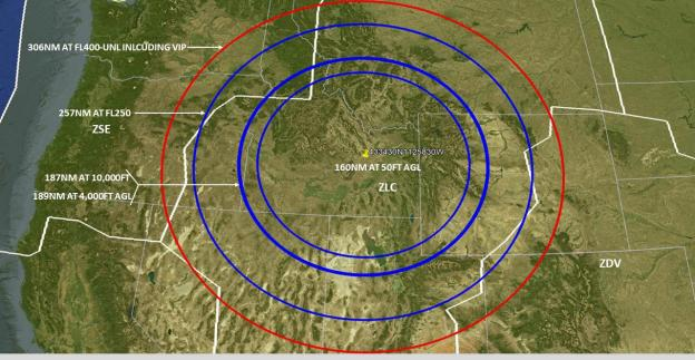
NATLID GPS 23-01 GPS INTERFERENCE TESTING NATLID GPS 23-01 GPS INTERFERENCE TESTING
