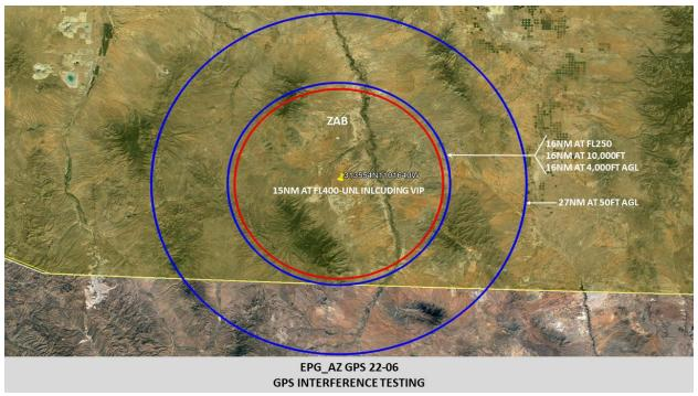
EPG\_AZ GPS 22-06 GPS INTERFERENCE TESTING
